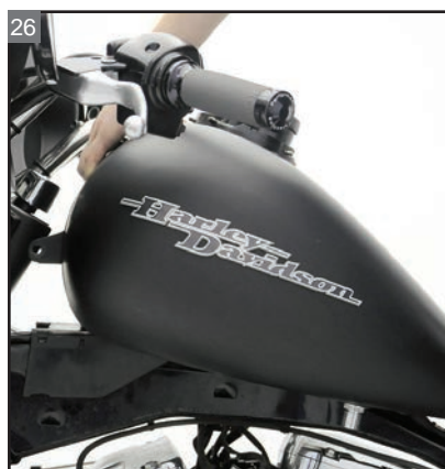
Install the tank onto the backbone.
