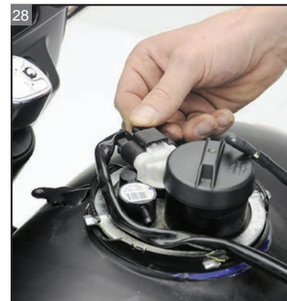
Plug in the fuel pump wiring.
