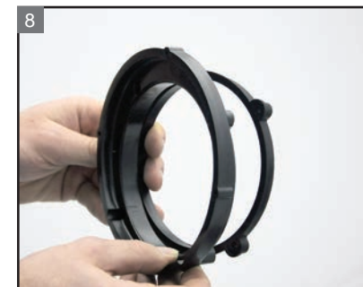
8 With a batwing fairing, stack the speaker adaptor rings like this.
