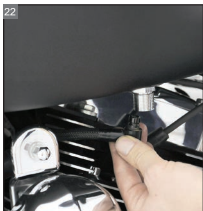
Disconnect the fuel line from the tank.
