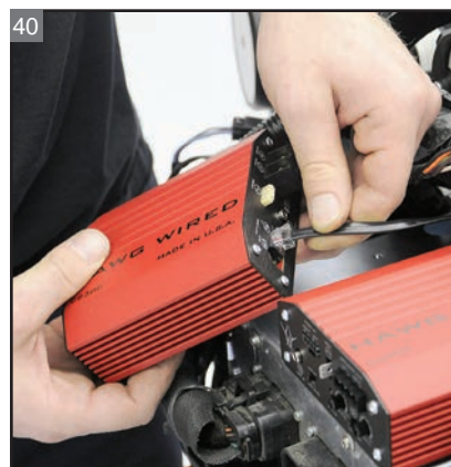
40 Plug the control wire from the other amp's OUT port into the IN port on the second amp.
