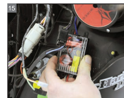
15 Remove the adhesive's backing and stick the crossover to the inner fairing.
