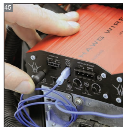
45 Plug in the LOW IN signal wire (this cable is from the back of the other amplifier).
