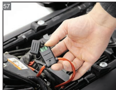
57 Install the fuses into the power wires.
