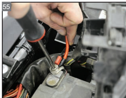
55 Install the amplifier power wires and tighten the battery bolt.
